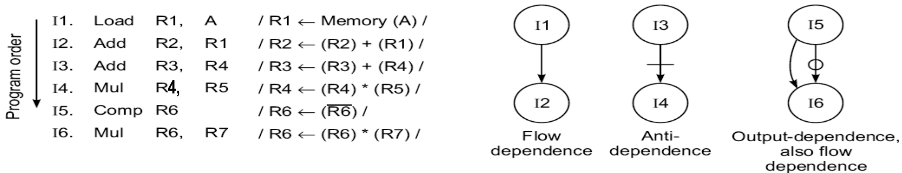
(b) A sample program and its dependence graph, where I2 and I3 share the adder and I4 and I6 share the multiplier
